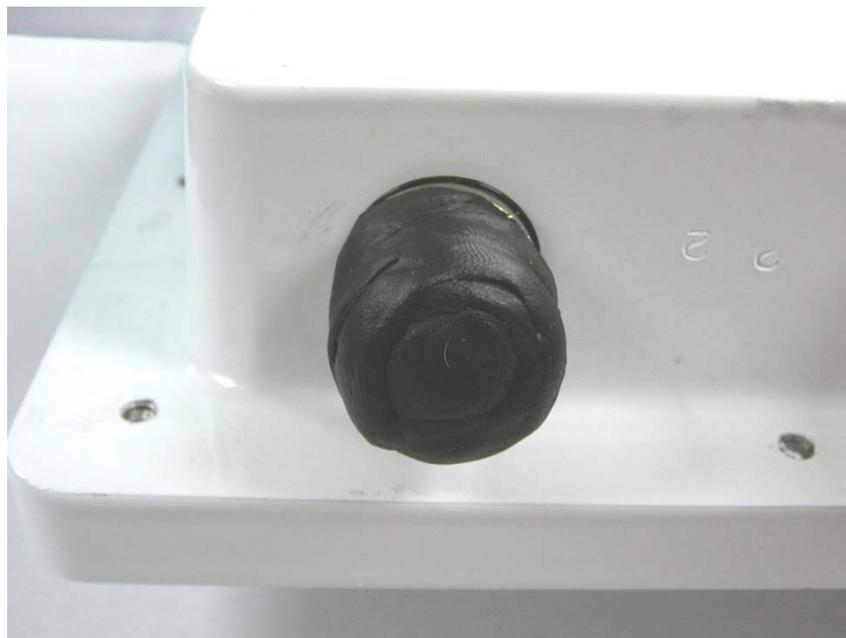
**Figure 2: Properly Taped External Antenna Port.**
