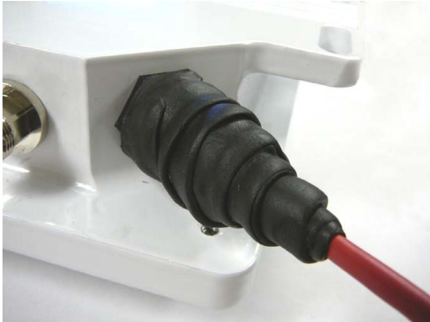
**Figure 1: Properly Taped Ethernet Connection**
